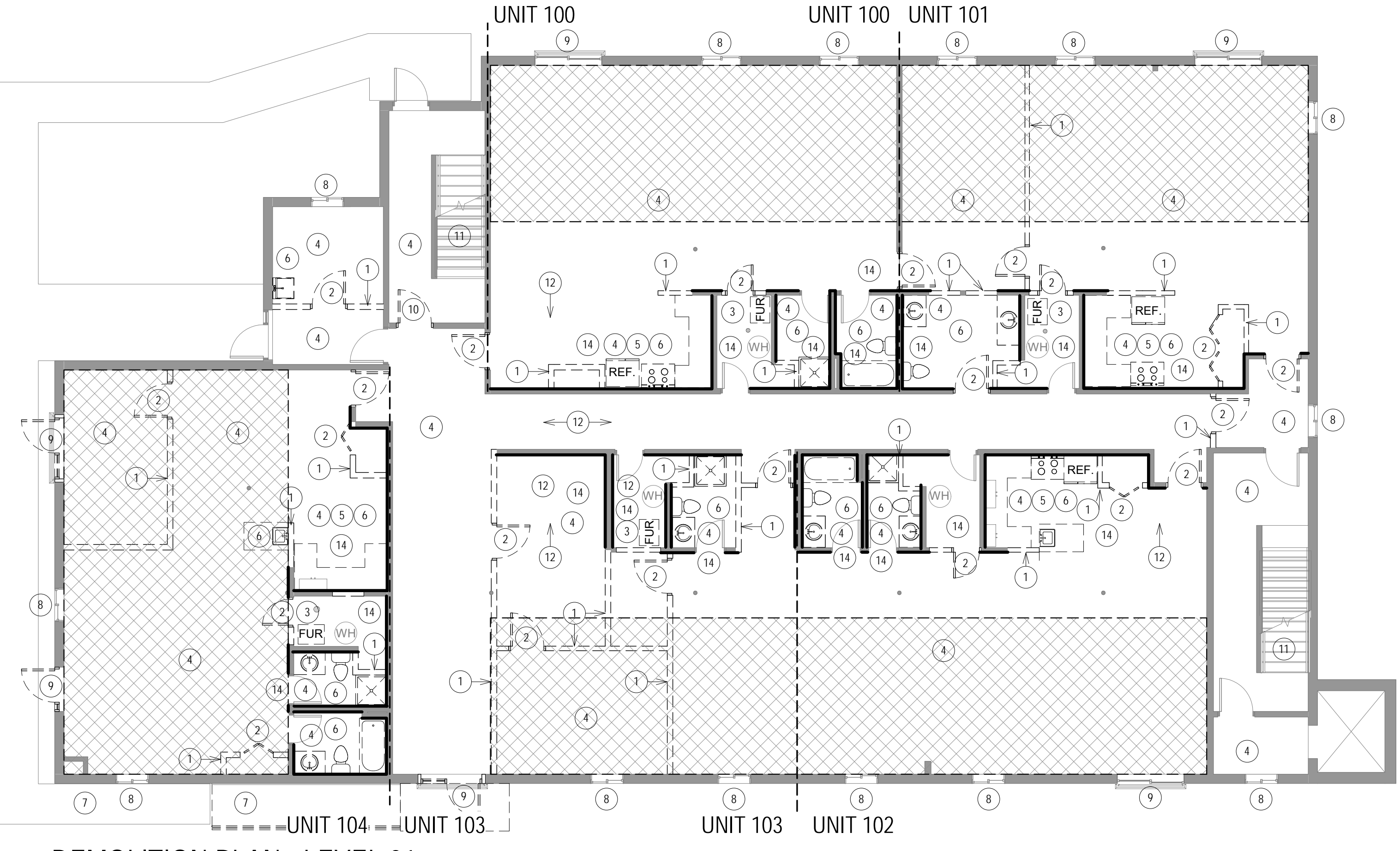
2 DEMOLITION PLAN - LEVEL 01 Scale: 1/8" = 1'-0"
