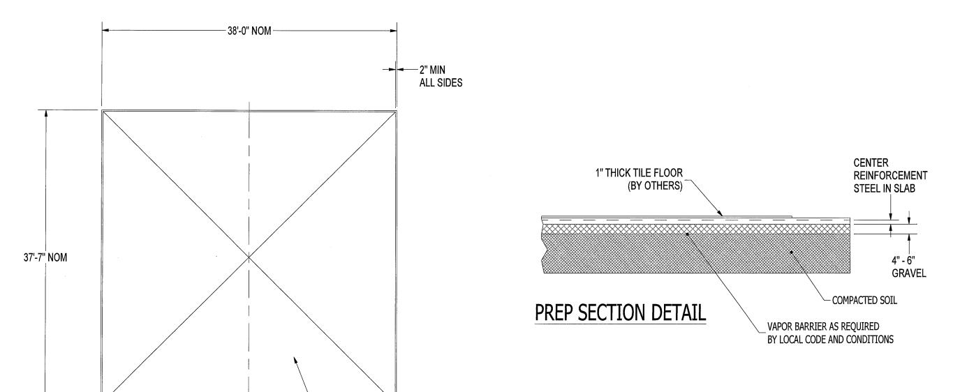
REINFORCING TO BE 6 X 6 X 6/6 WELDED WIRE MESH (WWM) PLACED IN THE CENTER OF THE SLAB TO EXTEND THROUGH ENTIRE - SLAB. UTILIZE SUFFICIENT NUMBER OF CHAIRS TO MAINTAIN WWM POSITION.
